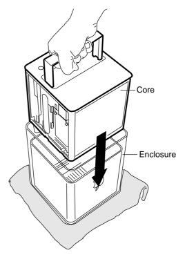
With a flat hand, press down on the latch until it locks into place. Firmly press the core to ensure it is fully secured within the enclosure.
